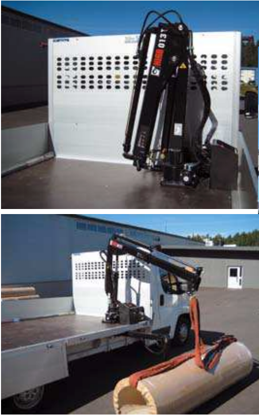
Hiab crane mounted on an aluminium platform for easier handling of goods. The crane is mounted on the right front of the bed with manual or hydraulic support legs.
