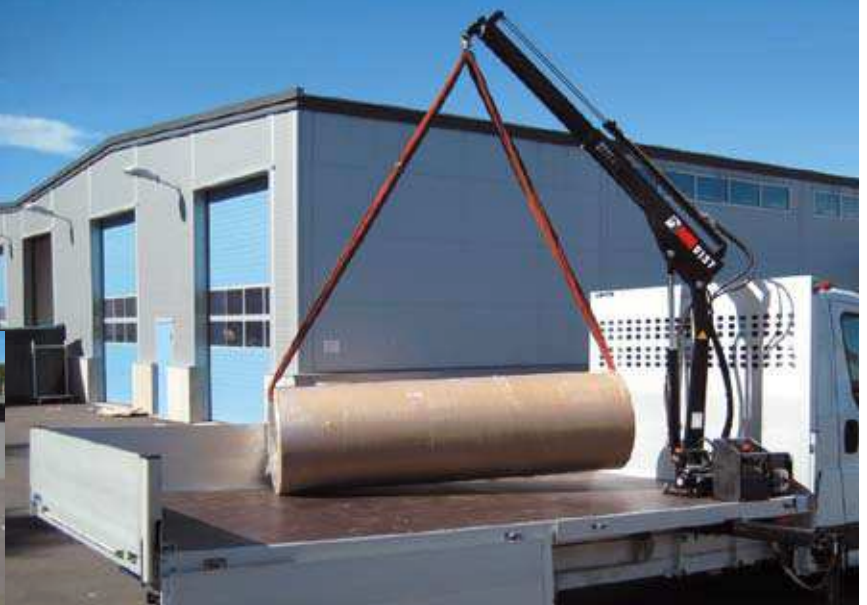
Hiab crane mounted on an aluminium platform for easier handling of goods. The crane is mounted on the right front of the bed with manual or hydraulic support legs.
