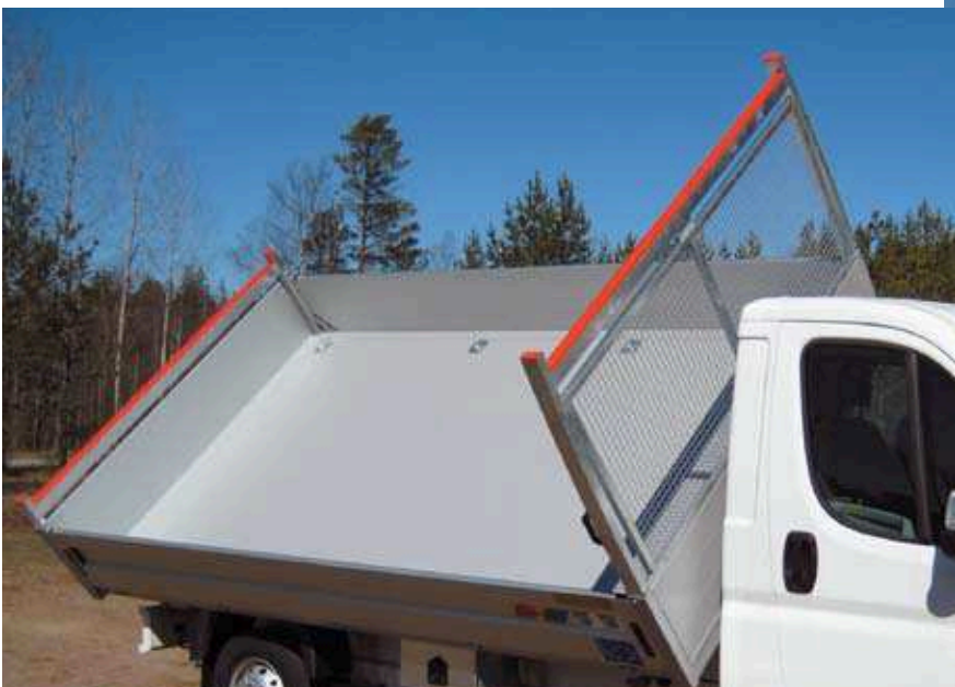
3-way tipper mounted on the chassis. The bed bottom and frame are in grey powder coated aluminium. The sideboards are constructed out of natural anodised aluminium. Load grating and middle frame are made from galvanised steel. The bed weight is approx. 480 kg depending on the model and size.
